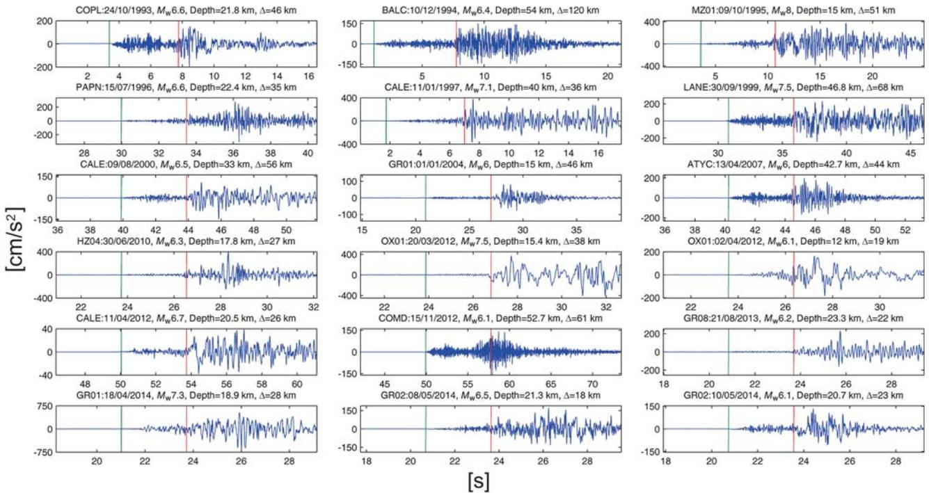
**Figure 3.** Strong-motion records of selected earthquakes analyzed in this study. The green and red tick marks show the arrival time of the  $P$  and  $S$  waves identified by the  $2(t_S-t_P)$  algorithm.
