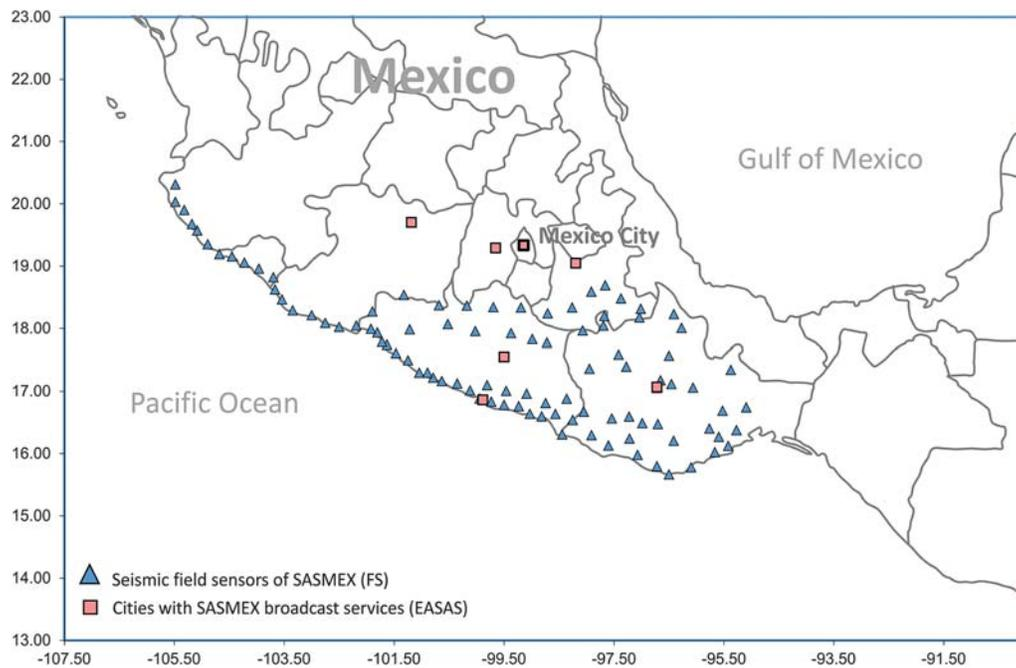
**Figure 1.** Current distribution of Seismic Alert System of Mexico (SASMEX) strong-motion stations (triangles) and alternate emitters of seismic warnings designed to disseminate the alert in various Mexican cities (squares).
