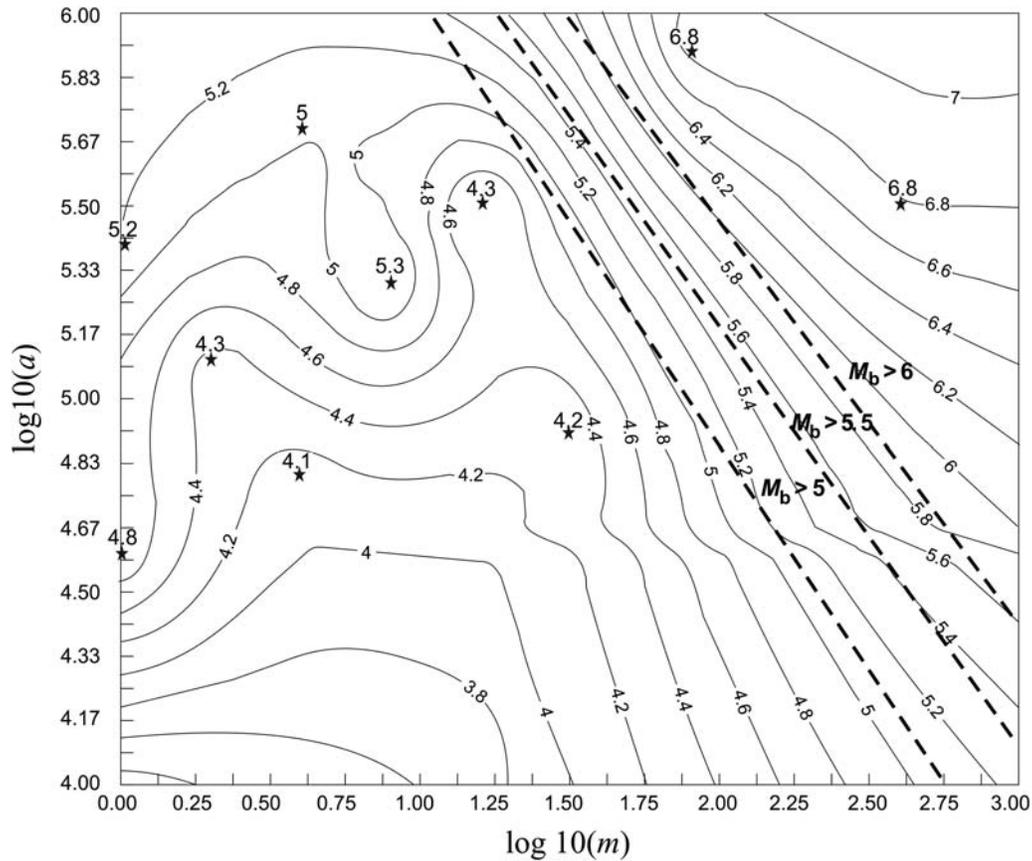
**Figure 5.** Magnitude  $m_b$  contours based on the parameters  $a$  and  $m$ . The calibration curves were estimated based on the data from 12 earthquakes occurring from 1985 to 1989, for which the epicenter lies at a distance of less than 80 km from the closest seismic sensors of the Guerrero strong-motion network (Anderson and Quaa, 1988).
