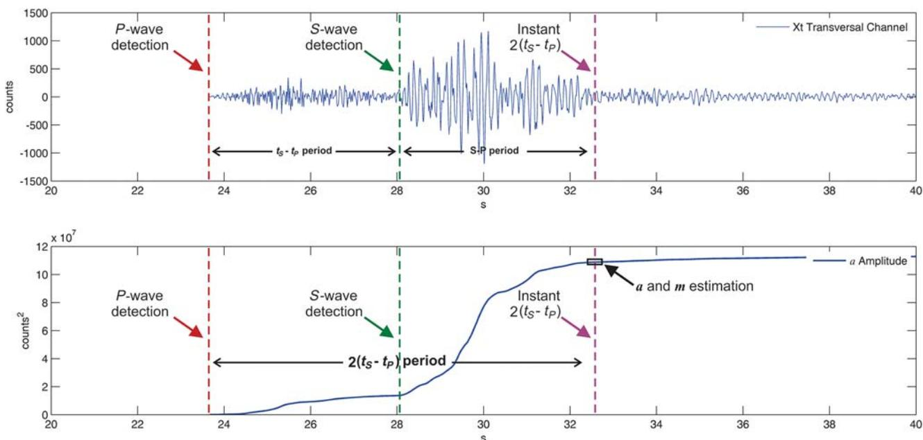
**Figure 4.** The upper trace shows an accelerogram of the 13 April 2007  $M_w$  6.0 earthquake. The box below shows the resulting function of the estimated quadratic amplitude  $a$  and instant rate of growth  $m$  calculated in the time period  $2(t_S - t_P)$ . The black arrow shows the time  $2(t_S - t_P)$  when the parameters are calculated.
