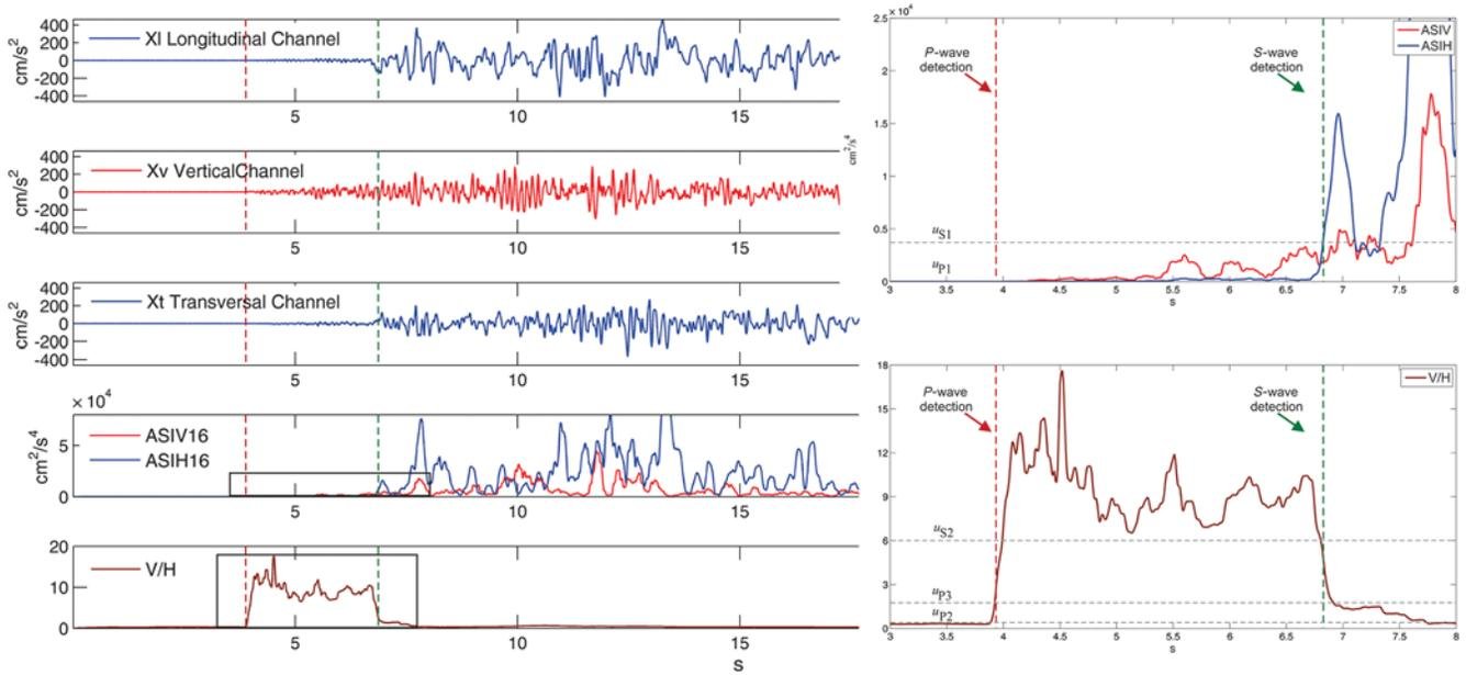
**Figure 2.** Example of  $P$ - and  $S$ -wave detection based on the  $2(t_S-t_P)$  algorithm. The first three traces show accelerograms from station Cacalutla for the 13 April 2007  $M_w$  6.0 Atoyac, Guerrero, Mexico, earthquake. The two lower traces show the characteristic functions used for detecting  $P$  and  $S$  waves, which are amplified in the box.
